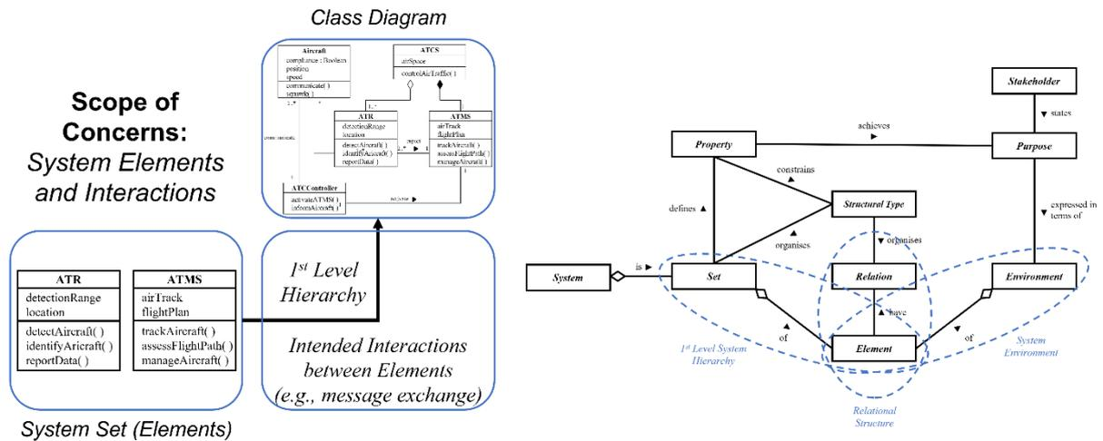
©Figure 6.11 Specification of system structure model [1]
