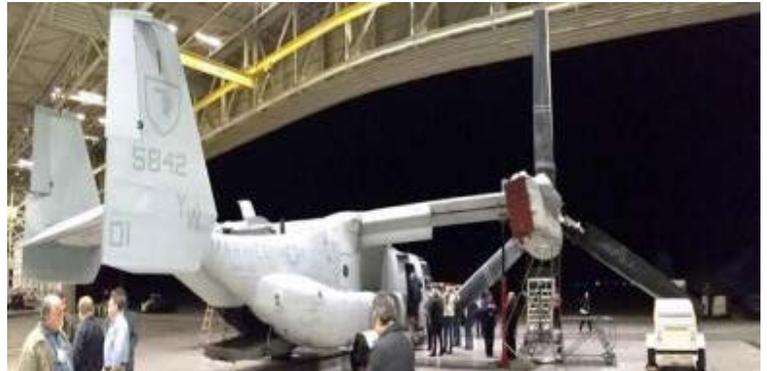
OMG Chairs toured the Osprey aircraft at the Marine Corps Air Station Miramar in San Diego, California. The Osprey uses tiltrotor technology to take off, land and hover like a helicopter. Once airborne, it can convert to a turboprop airplane capable of high-speed, high-altitude flight.
